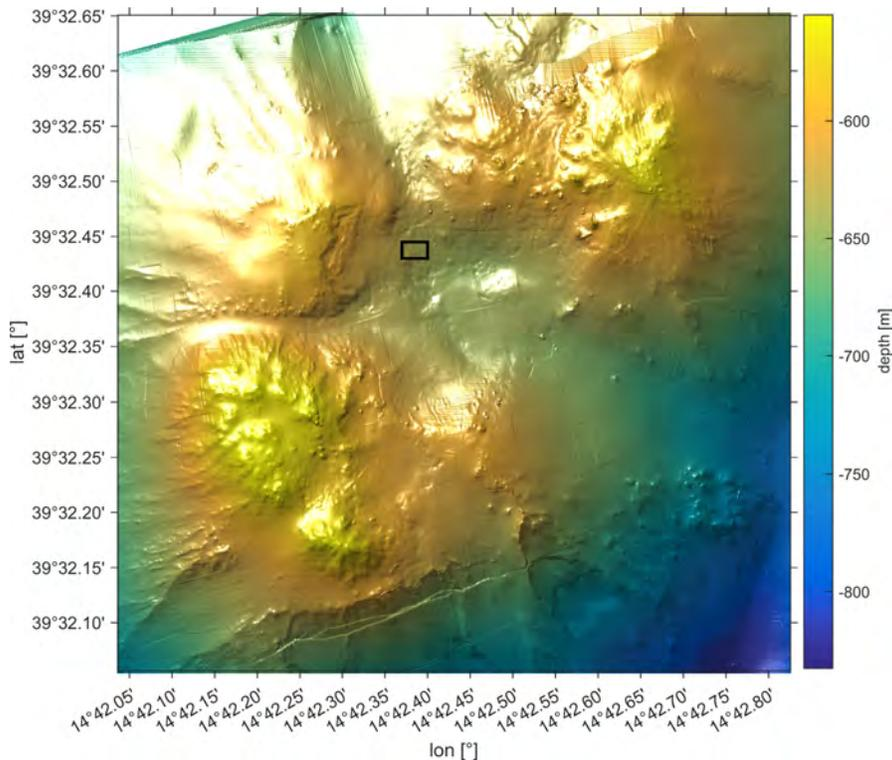
*Fig. 1: Bathymetric map based on AUV measurements at the Palinuro seamount (Petersen 2013). In several drillings (marked rectangle) massive sulfides were recovered in 2007 (R/V Meteor, cruise M73/2).*
