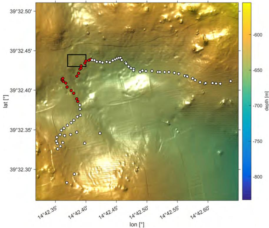
*Fig. 4: Bathymetric map of the Palinuro seamount with locations of TEM measurements (circles). Measurements at some locations showed significantly increased amplitudes (see Fig. 5), which are a strong indicator for the presence of conductive massive sulfides.*
