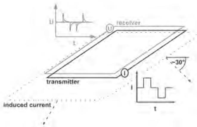
TEM systems usually use a bipolar waveform to generate a current in a transmitter loop ( Fig., black symbols),
