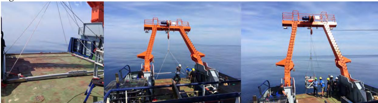
3: *TEM system with the 4.3m x 4.3m horizontal coil before deployment (left) and during deployment (middle) over the A-frame. After lowering of the coil into the water it was attached to a structure (right) holding the transmitter, receiver and the components.*
